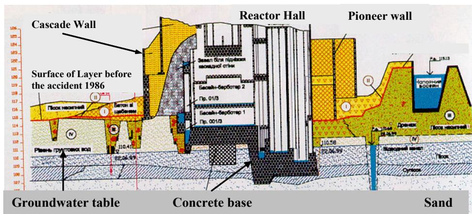
FIG. 6.2. Cross-section of the Chernobyl Unit 4 and the Shelter.
