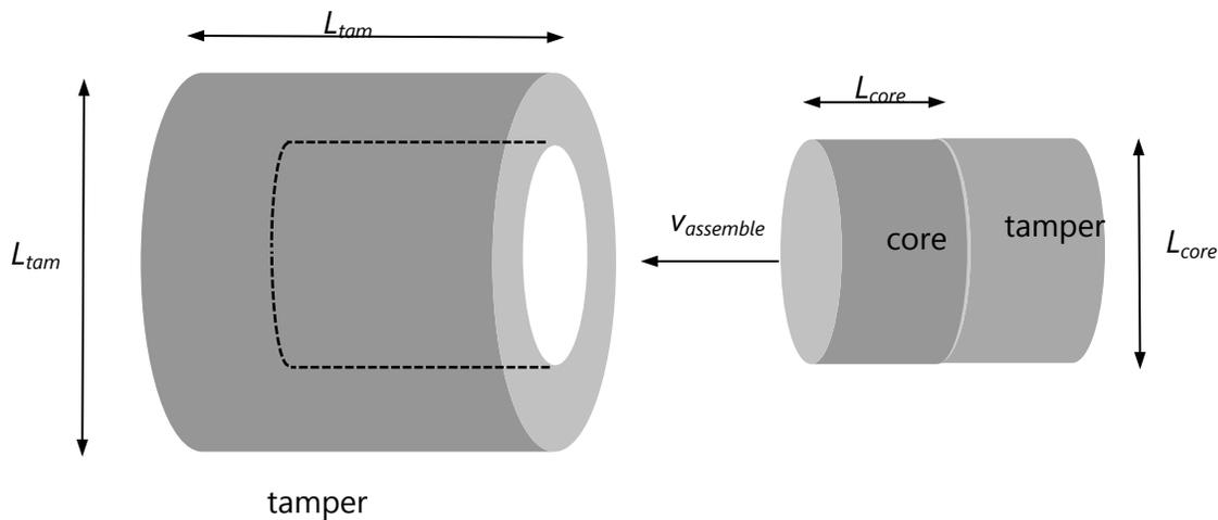
**Figure 1:** Sketch of a cylindrical tamper case and core/tamper-plug projectile assembly. A 40-kg U-235 core of normal density will have  $L_{core} = 14$  cm.
