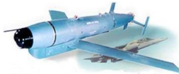
The H2 (Raptor) glide bomb, developed by South Africa, was its primary nuclear weapons delivery system. 60 km range.
