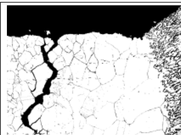
Figure 1: Intergranular stress corrosion cracking (IGSCC) in the sensitized heat-affected zone adjacent to a weld in Type 304 SS piping in a BWR (Source: Structural Integrity Associates, Inc., www.structint.com/tekbrefs/sib96154/ ).
