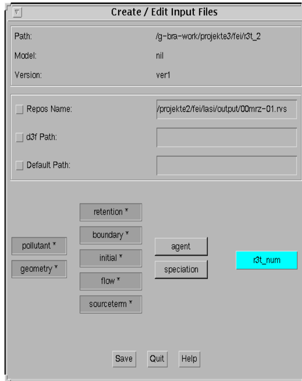
Fig. 6.3 “Create/Edit Input” window of preprocessor with switch to numerical control parameters
