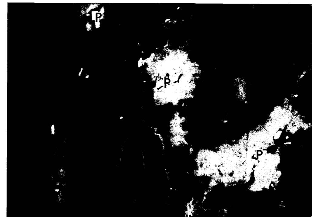
Figure 6 a. Anneal of colloids produced by dislocation wall migration ("dry" recrystallization). Note however, that these bleached areas can contain polyhalite (P). Asse Speisesalz (T41 Sp-800). Irrad. cond.: 100^\circ\text{C} , 15\text{ kGy/h} , 15.9\text{ MGy} . Mag. 34\times
