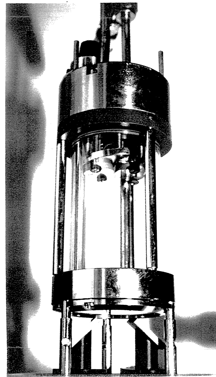
Figure 3 : Cell developed for FTIR spectroscopy
