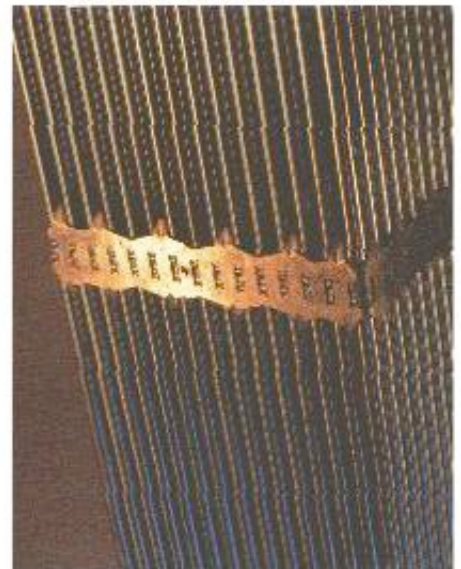
Figure 1: PWR fuel element
