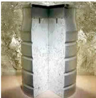
Cementation through the use of specially formulated grouts provides the means to immobilise radioactive material that is on solids and in various forms of sludges and precipitates/gels (flocks) or activated materials.
