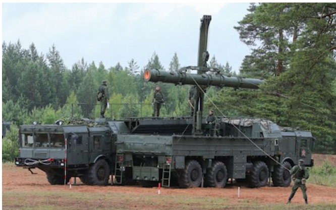
Possible Iskander-K GLCM canister transfer at Luga missile garrison, June 2014. Image: Russian MOD via Kristensen/FAS
